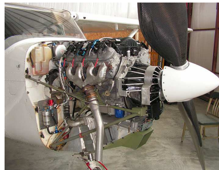
Above, this experimental configuration Cessna 172 has been re-engined with a 400hp Corvette LS1 V8 engine driving a large composite propeller. While certainly powerful it is not as light as an equivalent power DBR engine could be.
